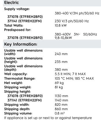
If appliance is set up or next to or against temperature sensitive furniture or similar, a safety gap of approximately 150 mm should be maintained or some form of heat insulation fitted.
